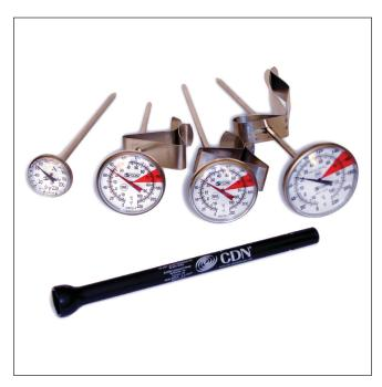
Recalibration is easy with the new Recalibration Tool on Sheath. Just immerse the thermometer in sheath in at least two inches of ice water, and then use the calibration tool to adjust the hex nut beneath the dial to 34°F. Recalibration can also be accomplished by immersing it in boiling water and adjusting to the appropriate temperature.
