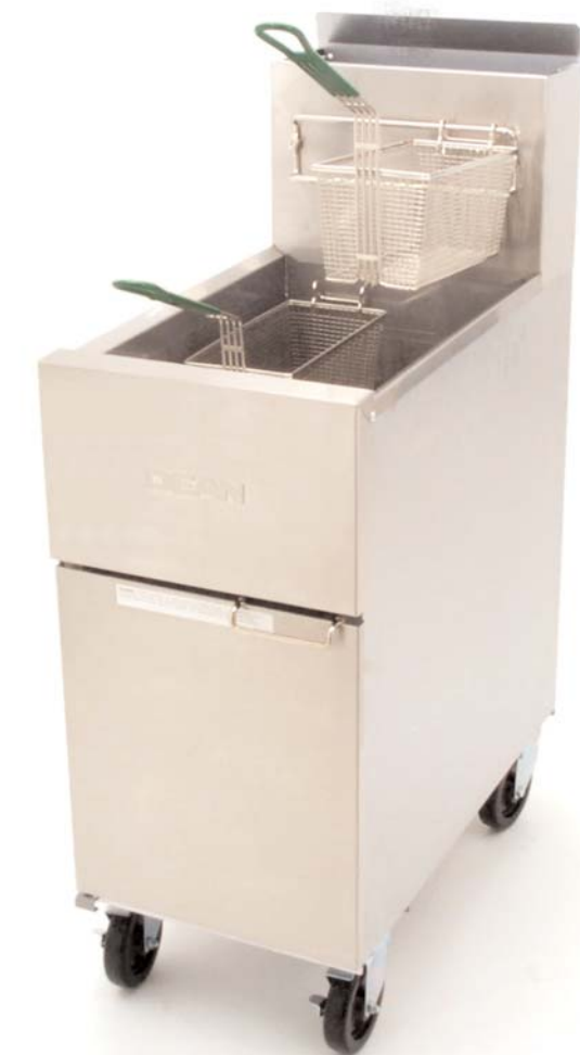
SR52G gas fryer standard with 120,000 BTU (30,600 kcal/hr.) (35.2 kW) burners and 50 lbs. (28 L) oil capacity. Shown with optional casters.
