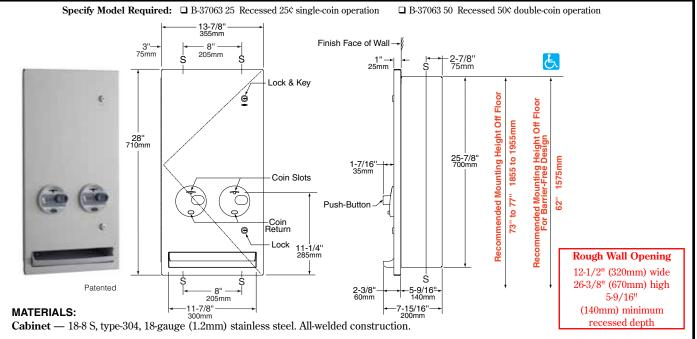
**Door** — 18-8 S, type-304, 18-gauge (1.2mm) stainless steel with satin finish. Door has flat design with 90° return edges; conceals flange. Secured to cabinet with a concealed full-length stainless steel piano-hinge. Equipped with two tumbler locks keyed like other Bobrick washroom accessories. Door has no brand-name advertising for products dispensed. Graphic symbols identify products dispensed and coin denomination.
