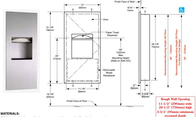
Cabinet — 18-8 S, type-304, heavy-gauge stainless steel. All-welded construction.
