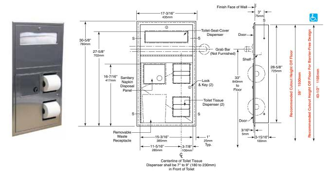
Rough Wall Opening 16" (405mm) wide 29-1/4" (745mm) high 4" (102mm) minimum recessed depth
